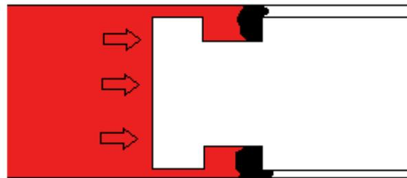
1. INCREASED PRESSURE FORCES THE O-RING TO EXTRUDE.
