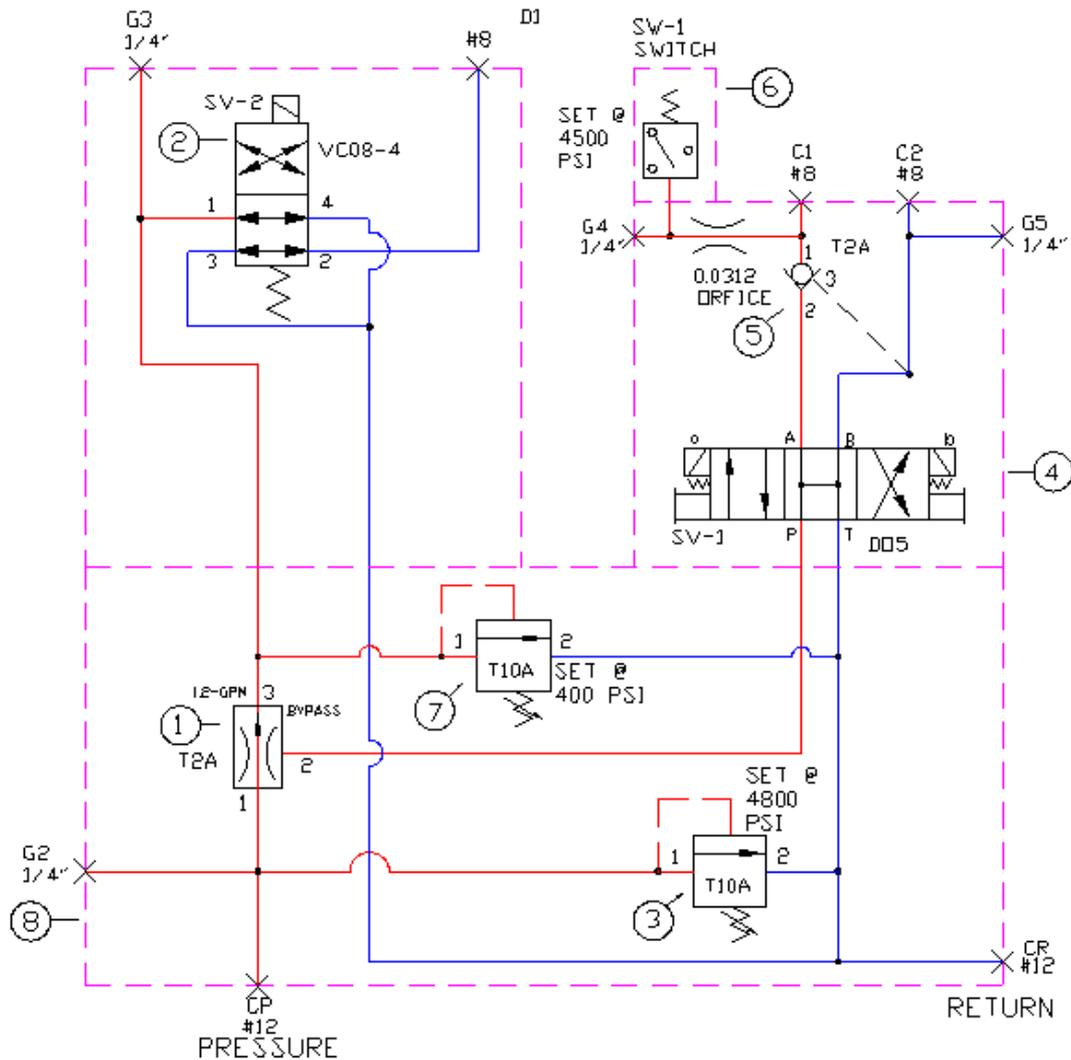
Item #5 is a pilot check valve used to trap hydraulic pressure on the closed side of the vibro clamp. There is also another one located right on the vibro clamp as well. If item #4 is in the center position, pump flow back to tank, then item #5 will trap any hydraulic pressure in the clamp close line to assure clamp remains closed.
