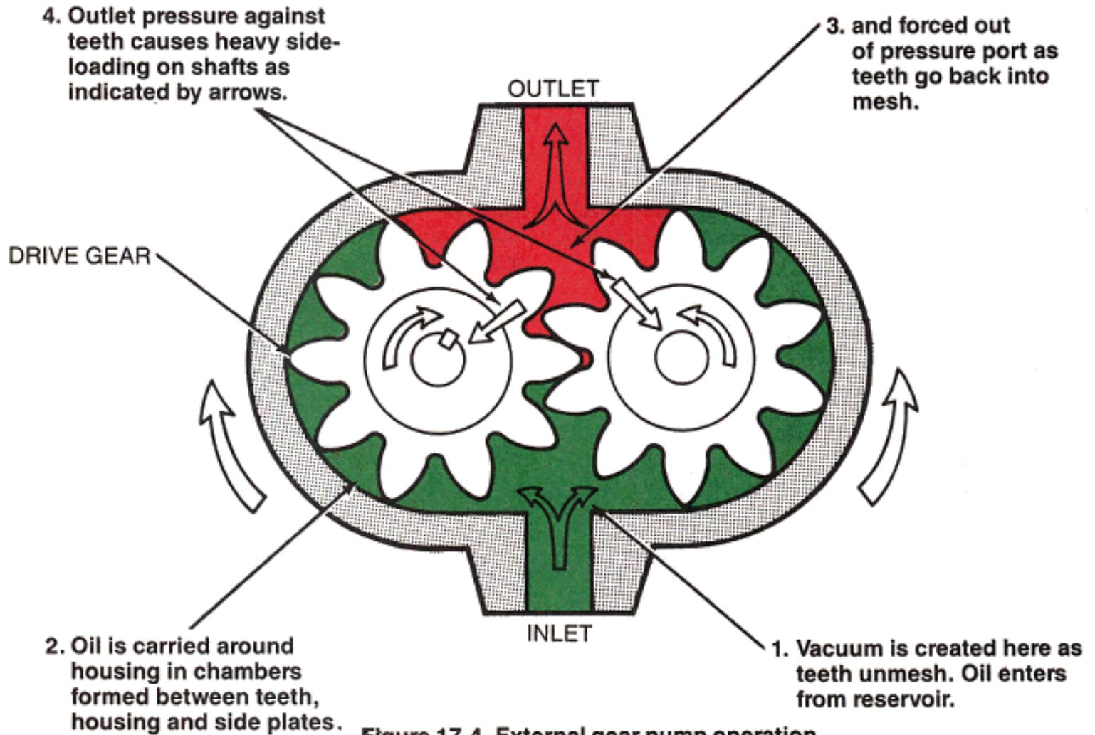
Figure 17-4. External gear pump operation.
