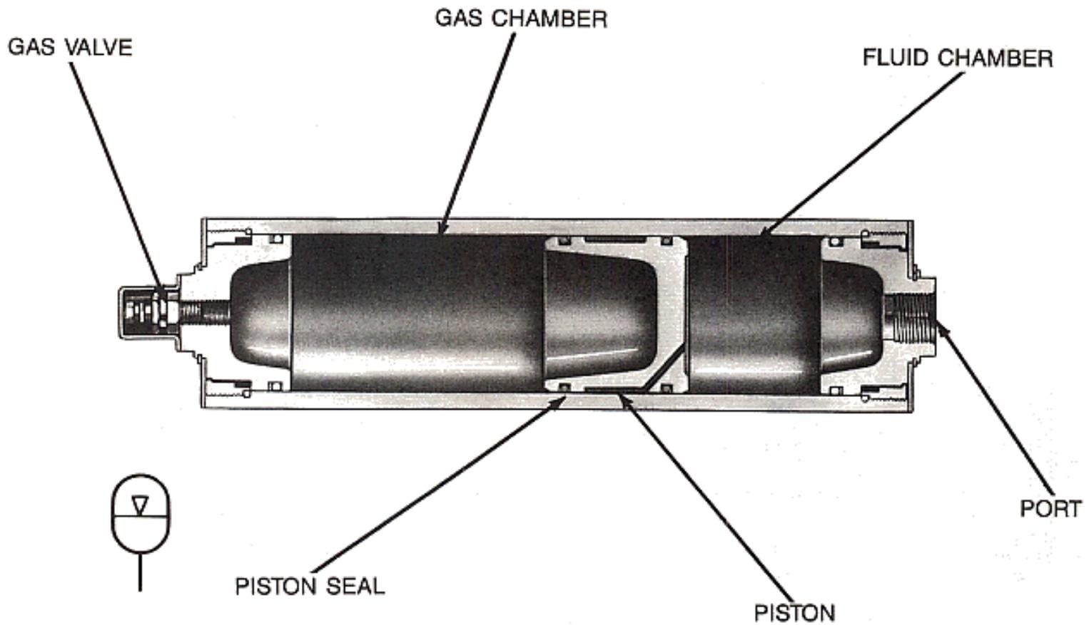
**Figure 18-3. Piston accumulator is gas-charged.**
