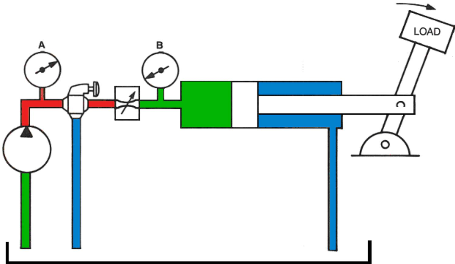
**Meter-In Circuits Do Not Control Runaway Loads**
