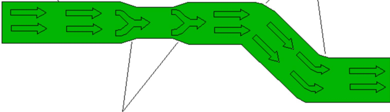
2. A gradual change in cross-section does not upset the streamline flow...
