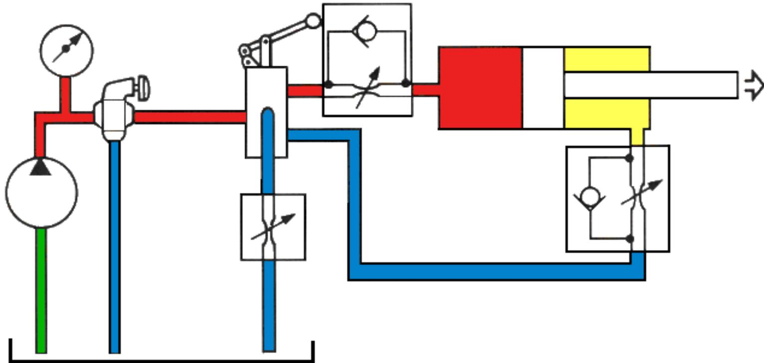
Colors based on piston extending and flow rate controlled by the rod-end valve
