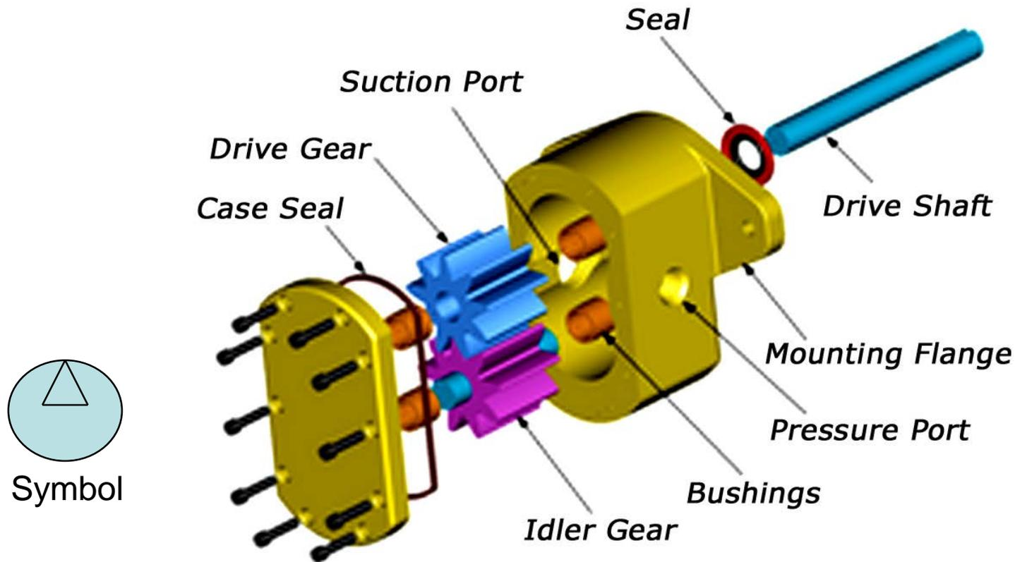
What does “fixed pump” mean? It means the pump displaces a fixed amount of oil per revolution. Much like a squirt gun. Squeeze the trigger and it pumps the same amount every time. This pump displaces the same amount every time it rotates. It pumps the moment the shaft turns and keeps pumping until the shaft stops. The faster you turn it, the more oil it displaces. You can slow down the output by slowing down the shaft speed. (turning down the rpm of the engine)
