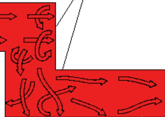
4. Nonparallel paths of particles increase resistance to flow (friction).
