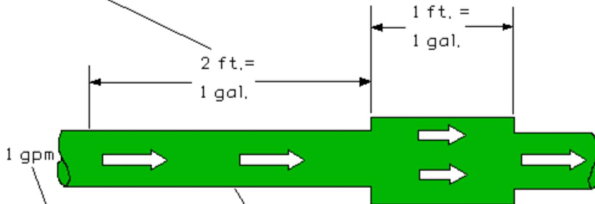
3. With a constant flow rate of one gpm...
