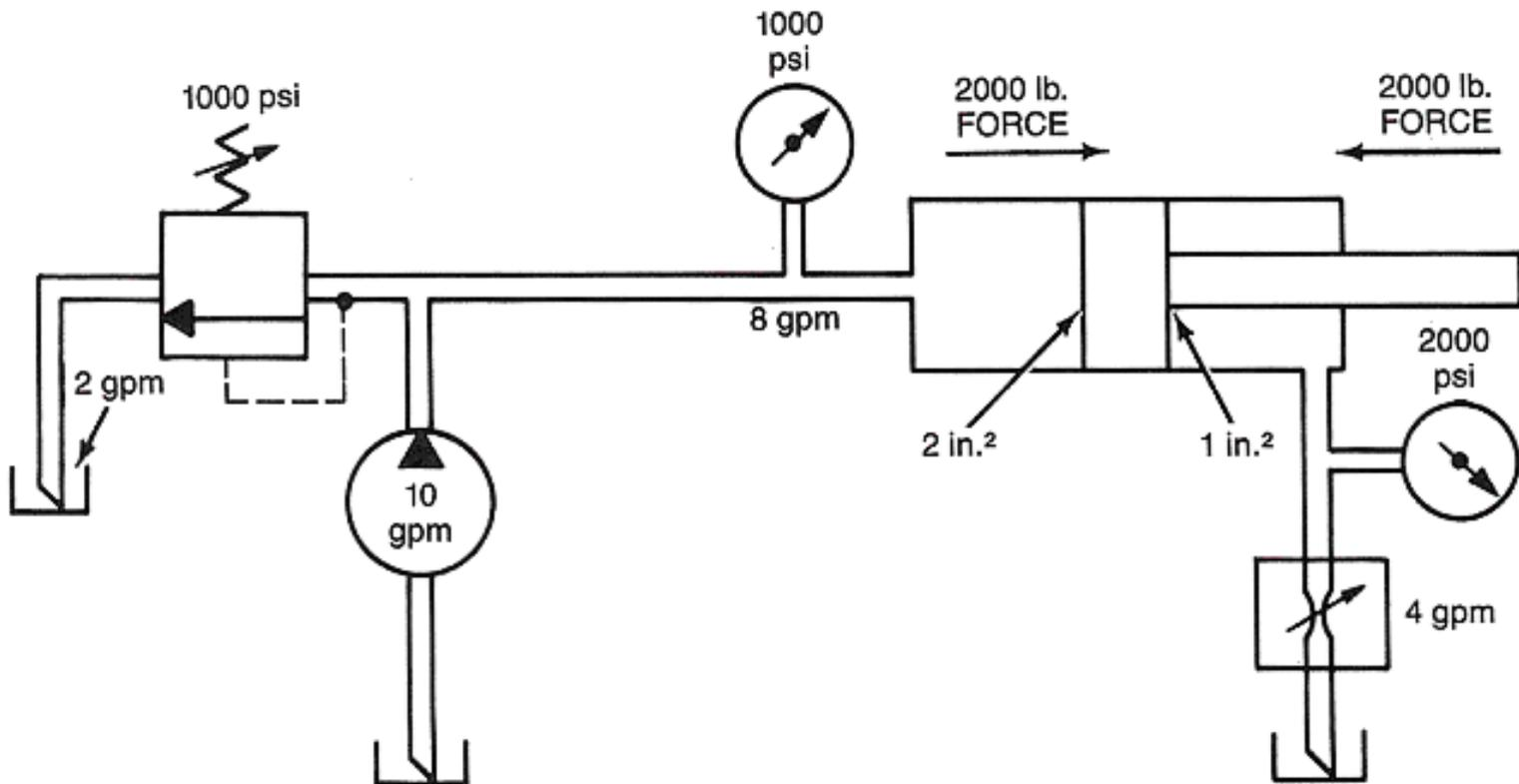
**Pressure Intensification in Meter-Out Circuits**
