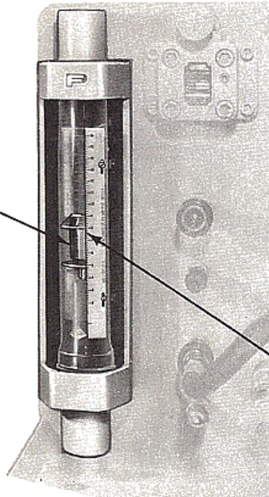
Flow rate in gpm is read directly on scale at this edge of indicator.
