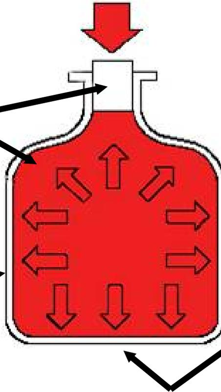
4. If the bottom has an area of 20 square inches and each square inch is pushed on by the 10 lb. of force, the entire bottom receives a 200 lb. push.
