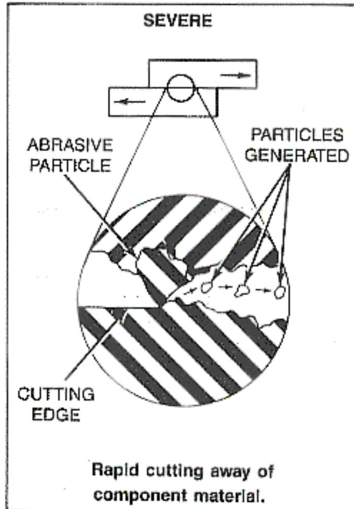
Mechanism of sliding wear with particles greater than the film thickness.
