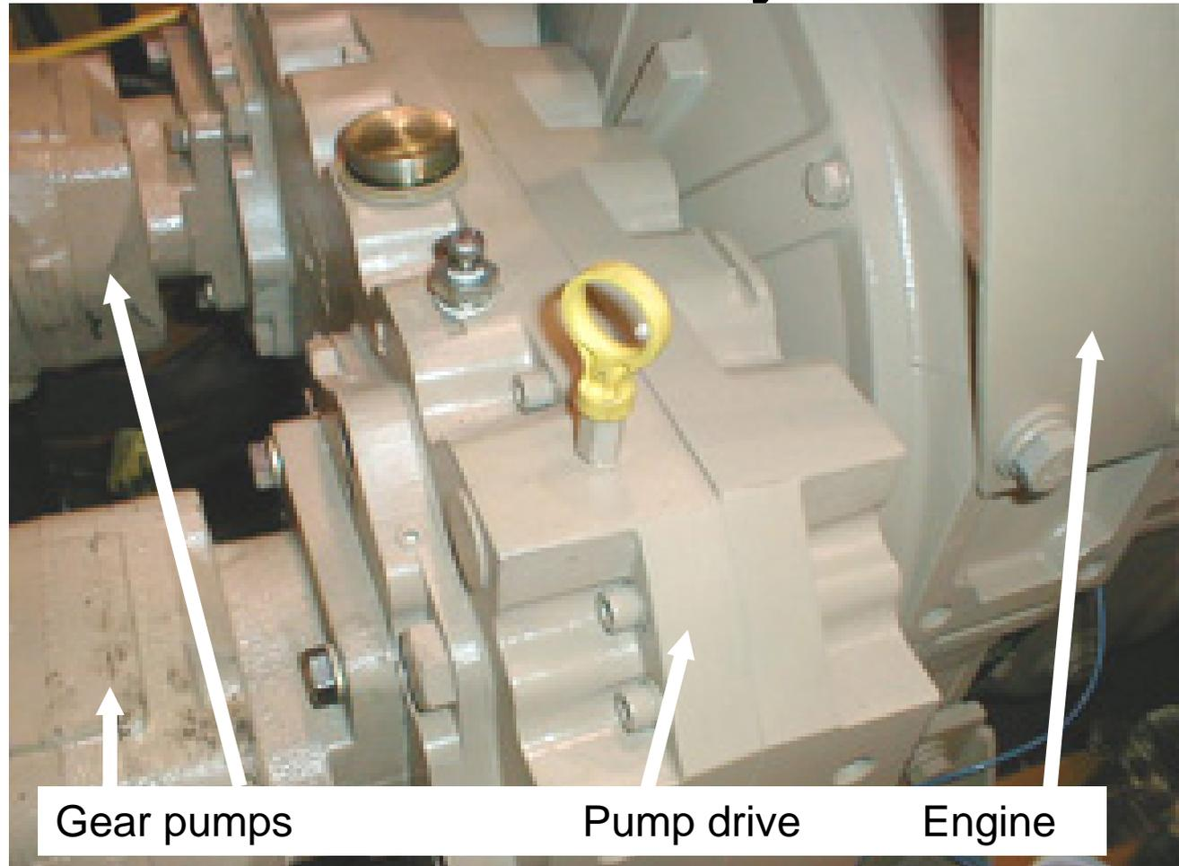
Do not always assume that the pump drive is turning at the same rpm as the engine. Ratios are stamped on the pump drive.
