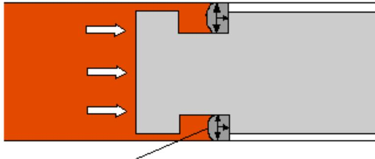
2. WHEN PRESSURE IS APPLIED, THE O-RING IS FORCED AGAINST A THIRD SURFACE CREATING A POSITIVE SEAL.
