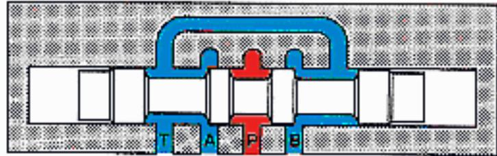
PRESSURED CLOSED—'A' & 'B' OPEN TO TANK
