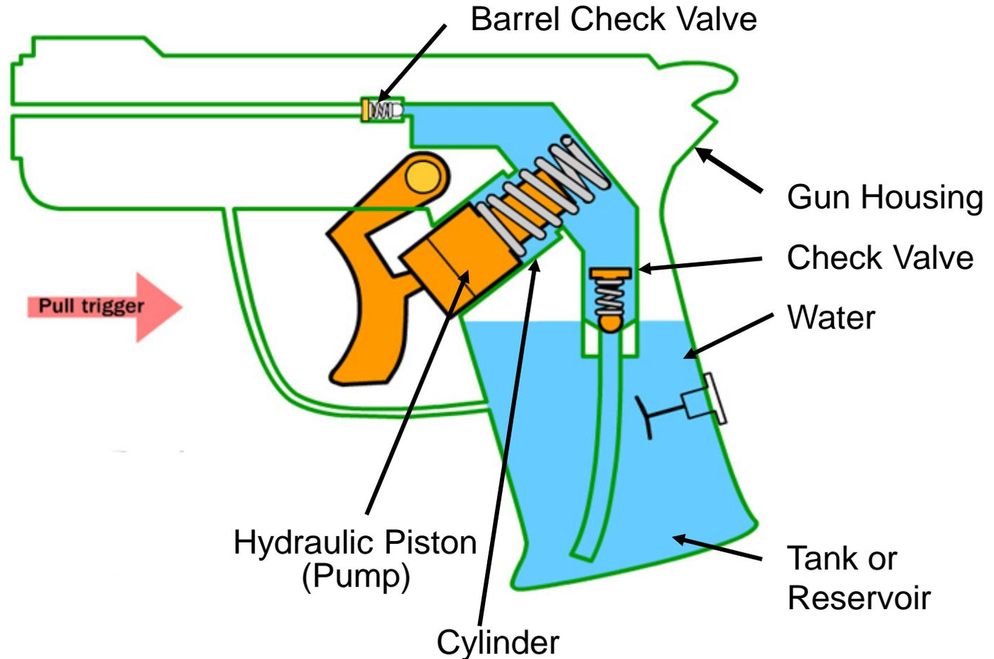
This is a simple check valve type hydraulic system just like our fuel pump on the diesel hammers; check valves that stop one direction and open in another. The injector on the diesel is really a check valve that works just like the check valve in the barrel of this squirt gun.
