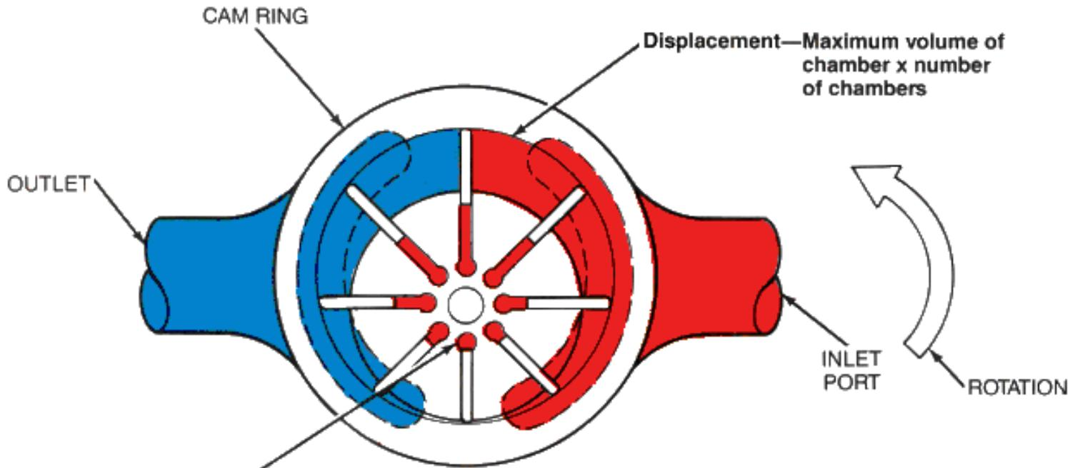
Displacement—Maximum volume of chamber x number of chambers
