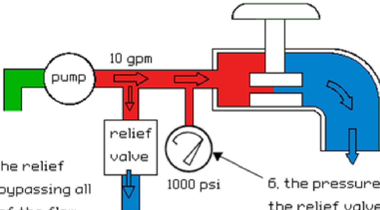
5. When the relief valve is bypassing all or part of the flow...
