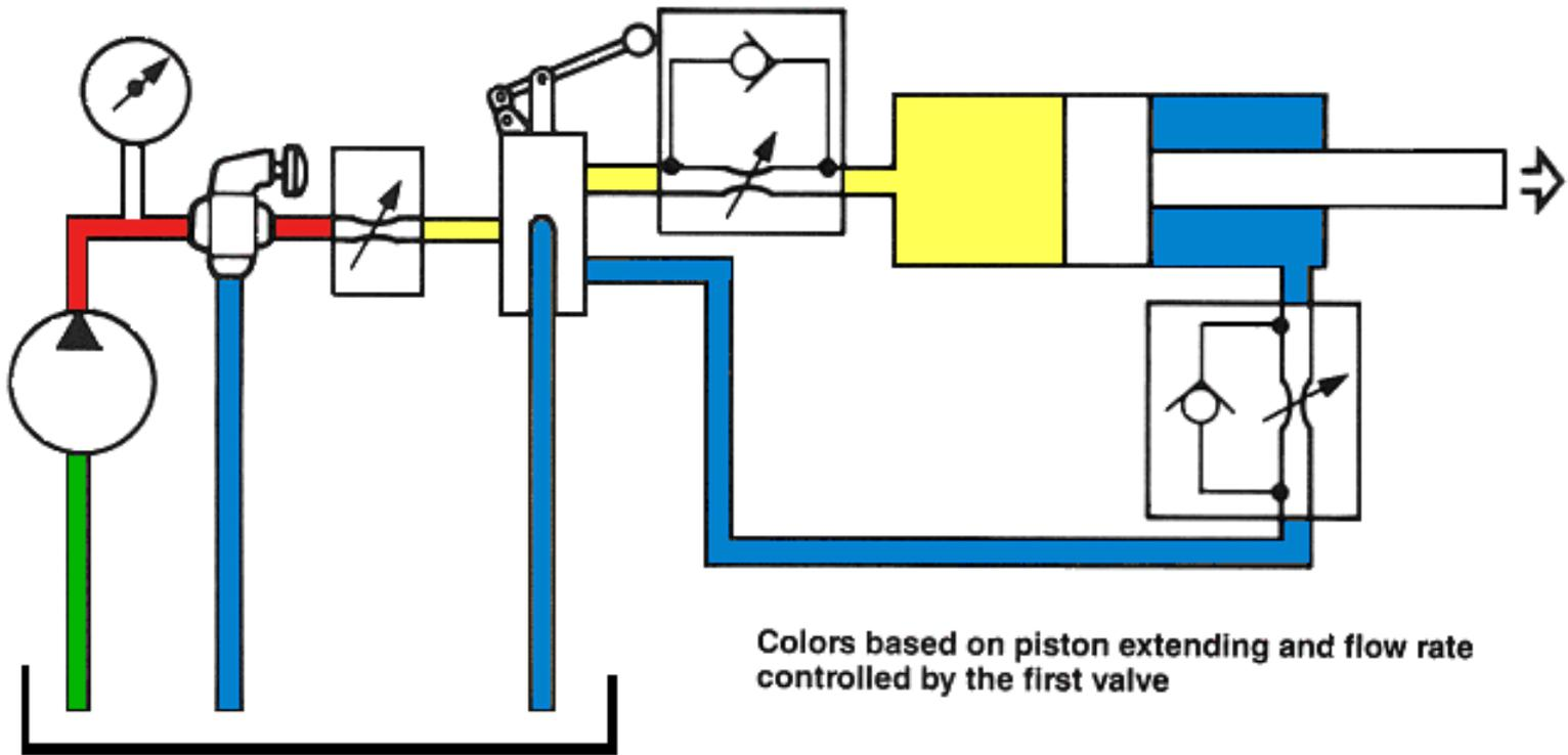
Colors based on piston extending and flow rate controlled by the first valve
