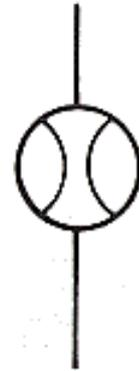
Figure 18-14. Typical flow meter.
