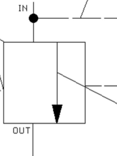
3. Arrow shows flow path and direction of flow.
