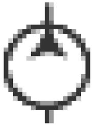
**Fixed Displacement Hydraulic Pump-unidirectional** (pumps only when rotated in one direction. Will not pump if turned backwards)
