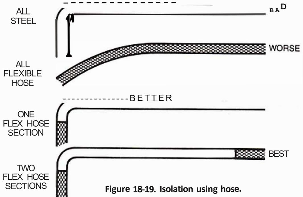
Figure 18-19. Isolation using hose.
