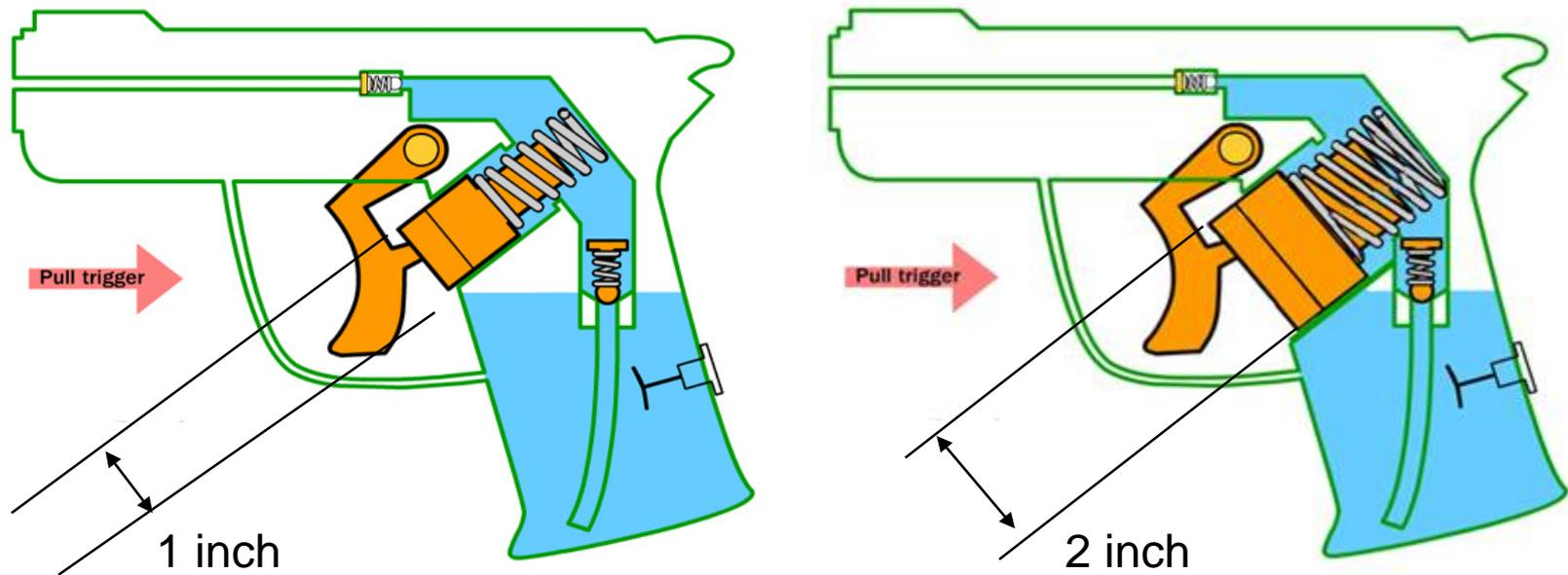
Changing piston diameter will increase volume of area. In this case, more water will be trapped in the cylinder on the gun to the right so it will spray more water per stroke. However, it will take more finger muscle to squeeze the one on the right, just as it takes more horsepower to increase pump output. Gear pumps increase with gear size, piston pumps increase with piston size or length of stroke or by adding more pistons.
