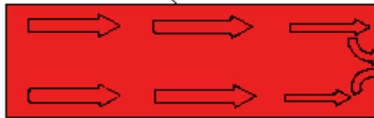
2. An abrupt change in cross-section makes it turbulent,
